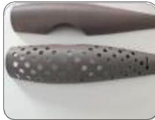
Fuselage of an aerial robot prototype by large-format AM using sustainable composite materials and advanced textiles
