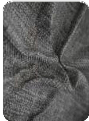
Bidirectional thermoplastic prepreg made out of recycled carbon and polyamide 6
